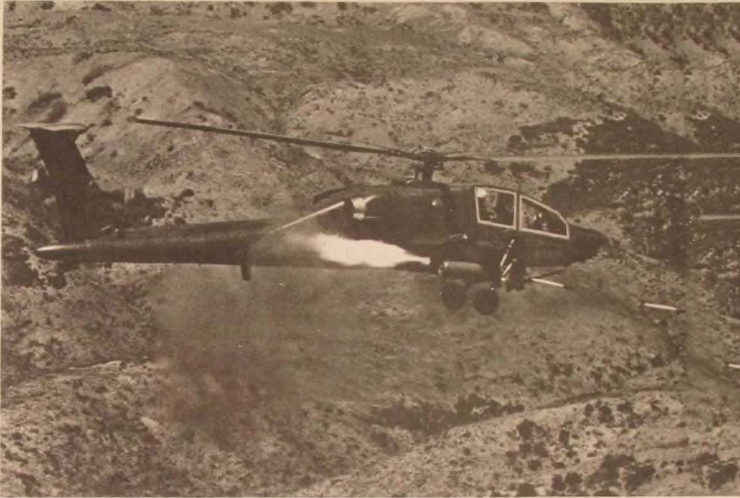
A heavily armored Hughes YAH-64 advanced attack helicopter fires 2.75-inch unguided, folding fin rockets in Army development and testing. These rockets come with a variety of warheads but are intended for use mainly against personnel and other "soft" targets. . . . The YAH-64 is intended by the Army to be a major antiarmor weapon system. Two YAH-64s (facing page) are shown in nap-of-the-earth flight with subwinglet pods designed to carry the HELLFIRE guided antitank missile. The flat windshield panels reduce solar canopy glint and render the helicopter less vulnerable to visual detection.
